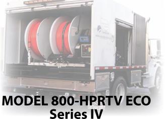
**System:** Integral to the 800-HPRTV ECO Series IV, this system is powered by Cues and comes complete with a self-leveling straight-view camera, color monitor, keyboard, footage counter, and a USB flash drive. All components are housed in a weather-rated enclosure, located at the jetting operator station.
