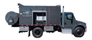
The exclusive ECO operating system combines with simplicity and efficiency of a PTO hydrostatic pump drive with a power plant that operates at lower RPM than traditional designs. Trucks equipped with ECO options experience less engine wear and lower fuel consumption, saving operators time and money.
